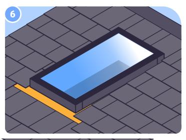
**Step 4** Install a timber batten (minimum 25mm wide) to support the roof light on the inside of the upstand kerb. The timber batten should be installed the correct height from the top of the waterproof layer on top of the upstand. (28mm for double glazed & 44mm for triple glazed).
