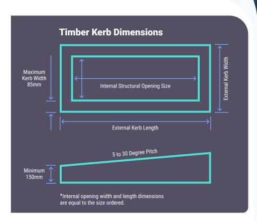
Example of a 5-degree minimum pitch: This equates to a grade of 1:11.5. E.g. a roof light with 1000mm width will require a fall of 87mm.
