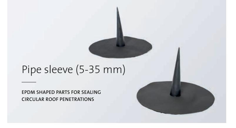
EPDM shaped part for slipping over and sealing in roof penetrations with a round cross-section and diameters of 5 to 35 mm. The connecting collar consists of a circular piece of RESITRIX® SK W Full Bond with a diameter of up to 30 cm.
