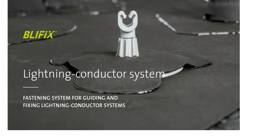
BLIFIX® is a fastening system for guiding and fixing lightning-conductor systems with maximum diameters of 10 mm on flat-roof constructions without ballast. The BLIFIX® holder system consists of a round plastic base plate, diameter 100 cm, with a plug-in and horizontally-alignable guide for the lightning-conductor system. BLIFIX® is fixed to the roof using a shaped part made of RESITRIX® MB, which can be slipped on and welded into place.
