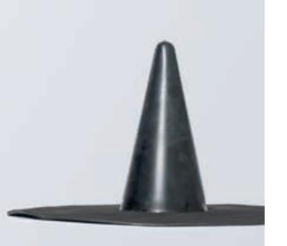
EPDM shaped part for slipping over and sealing in roof penetrations with a round cross-section and diameters of 35 to 100 mm. The connecting collar consists of a circular piece of RESITRIX® SK W Full Bond with a diameter of 50 cm.
